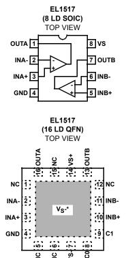
\*THERMAL PAD MUST BE CONNECTED TO NEGATIVE SUPPLY:  $V_S$ -QFN PACKAGE CAN BE USED IN DUAL SUPPLY APPLICATIONS.
